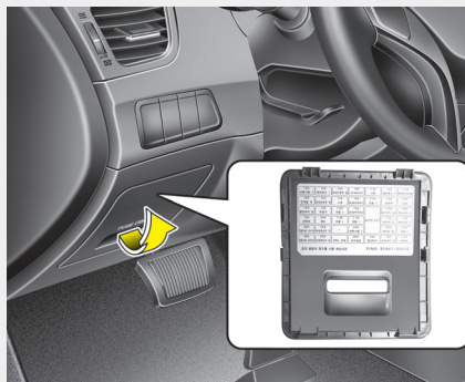
Inner panel fuse panel
